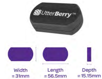
Fig. 27 a Original WSN system developed at the University of Cambridge in 2009, b tilt mote (Wisen innovation), c laser distance mote (Wisen innovation) and d displacement/acceleration mote (Utterberry)
