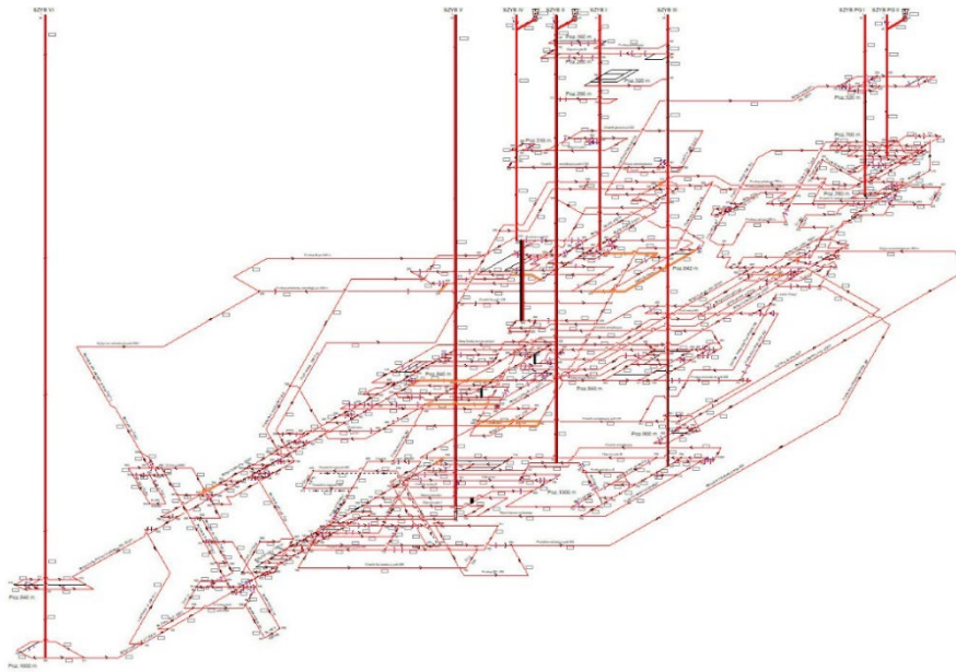
FIG 2 – Example 1 mine ventilation network scheme.
