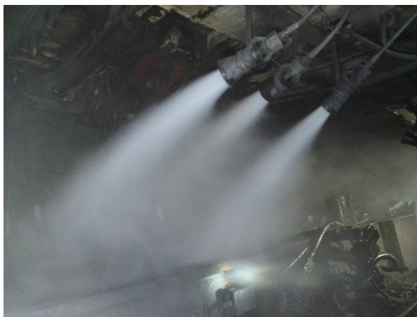
FIG 3 – Novel spray device of fully mechanised mining face: (a) Hydrodynamic fan spray device used in the coal cutter; (b) Negative pressure coiling device used in the fully mechanised mining shelf.
