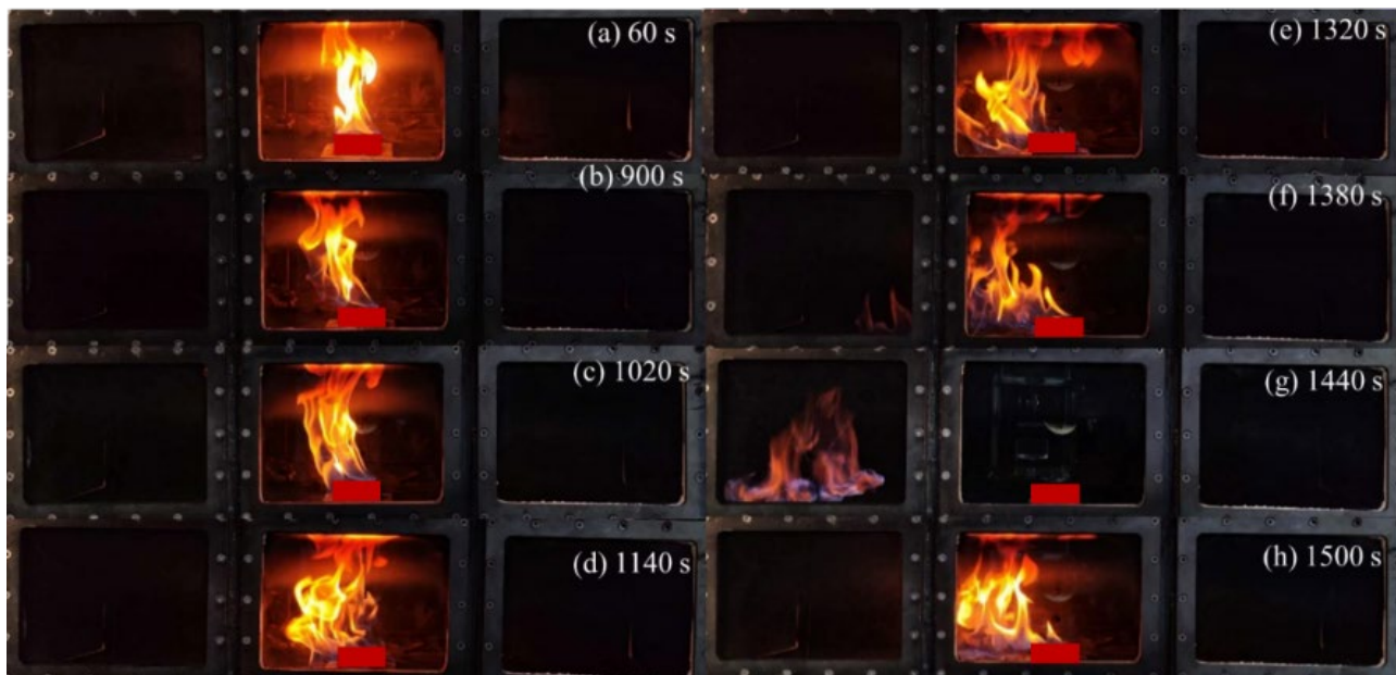
FIG 3 – Flame shapes (sealing ratio is 0).
