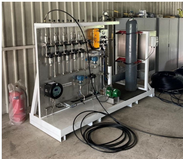
FIG 2 – Commissioned leak tester prototype.
