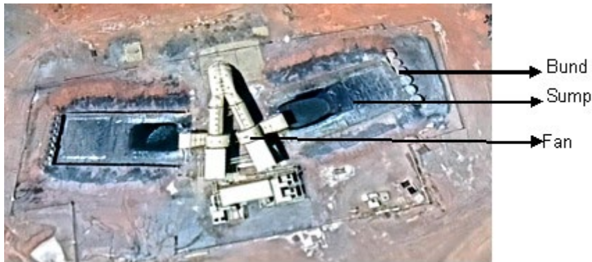
FIG 3 – Sumps with closed bund.
