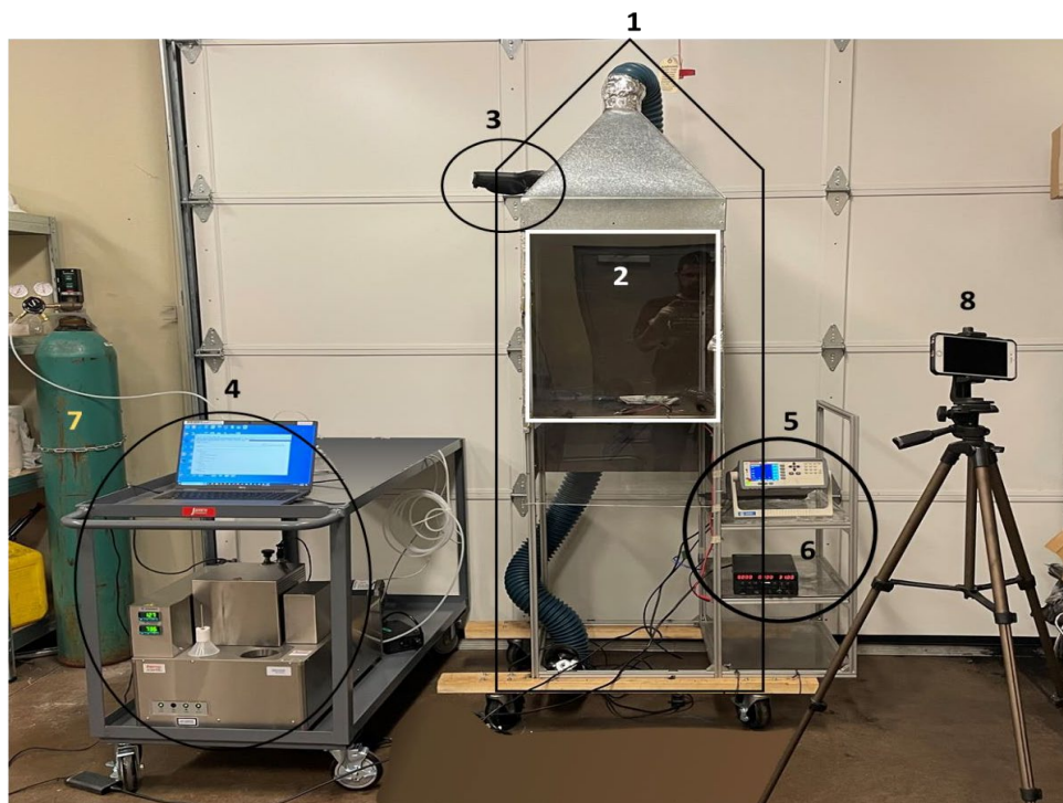
FIG 1 – Lithium-ion battery analysis system with; 1: LIB incinerator, 2: Fire Chamber, 3: Thermal Camera, 4: FTIR including a PC for gas analysis, 5: Thermocouple Data Logger, 6: DC voltage regulator, 7: Nitrogen Tank, 8: A mobile phone for video recording.
