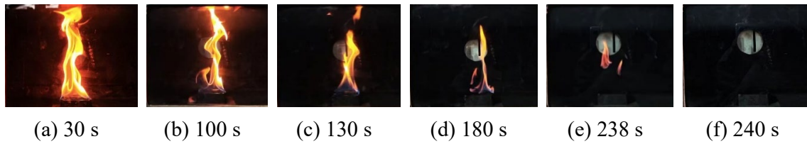
FIG 4 – Flame shapes (6 cm × 6 cm, upward sealing, sealing ratio is 70 per cent).
