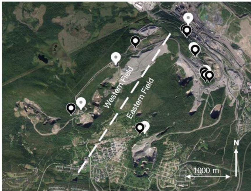
FIG 1 – Overview of the mining area division into the Western and Eastern Fields and the locations of the six intakes (white markers) and 11 exhausts (black markers).
