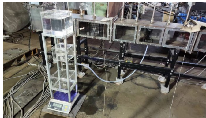
FIG 2 – Measurement point arrangement and Liquid-level stabilisation device: (a) Measurements positions; (b) Thermocouple tree; (c) Liquid-level stabilisation device.
