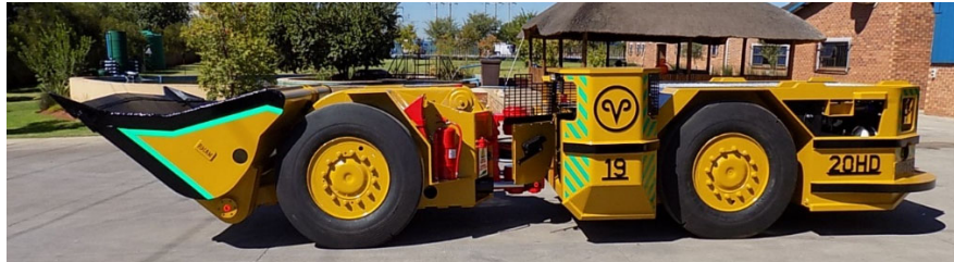
FIG 3 – Rham model 20HD low profile LHD ( https://miningtara.co.za ).
