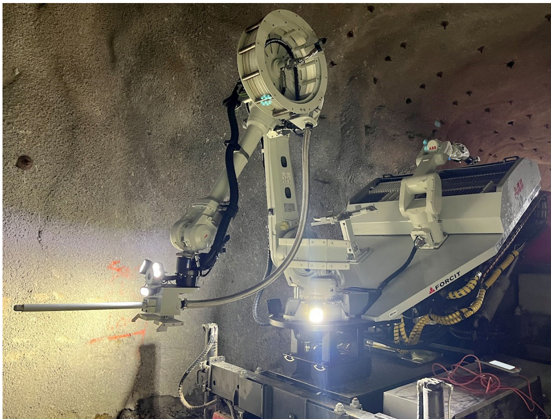
FIG 3 – The charging truck with the robot arms and the storage for bulk explosives and the detonators. The technology includes vision systems and automation solutions to communicate with the truck crane and ABB industrial robotic arm (image courtesy of ABB).
