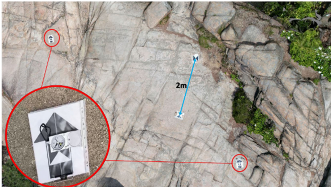
FIG 5 – Placement of ground control points (GCPs) for accurate rock mass mapping.
