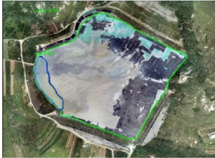
FIG 6 – The extracted contours delineating the beach interface and the boundary edge of the decant pond using the optimised YOLACT model.
