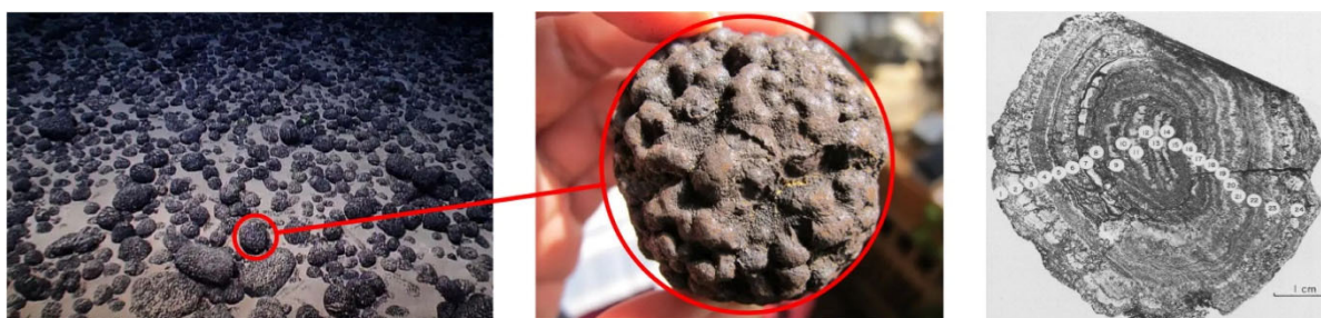
FIG 1 – Deep-sea Polymetallic nodules (left: appearance on seabed, middle: close up, right: cross) (Piper and Williamson, 1981).
