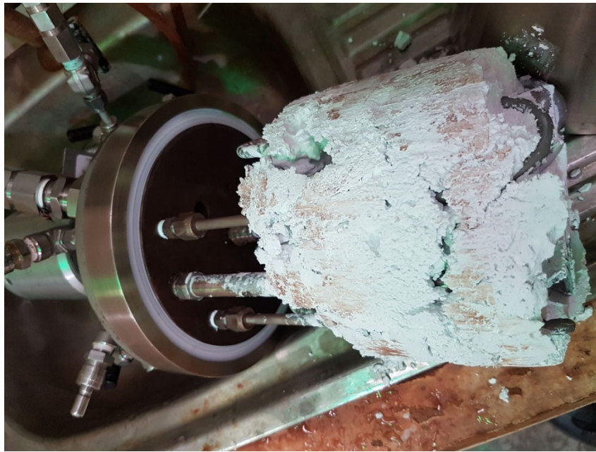
FIG 2 – Solid mass formed during Test 1 sticking to the autoclave impellers.
