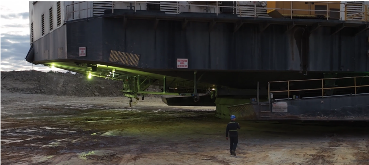
FIG 3 – Dragline Proximity Awareness being triggered by a person entering the operational zone during validation process/commissioning. Source: Coronado Curragh Pty Ltd. Not for further distribution or use.
