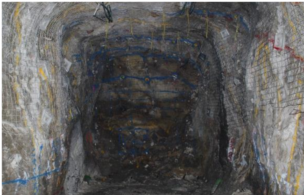
FIG 3 – 703 DP3 after charging face and rings showing tether tapes of pre-charged holes.
