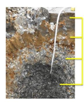
Zone 1 Sediment-sludge layer (~330 mm)
