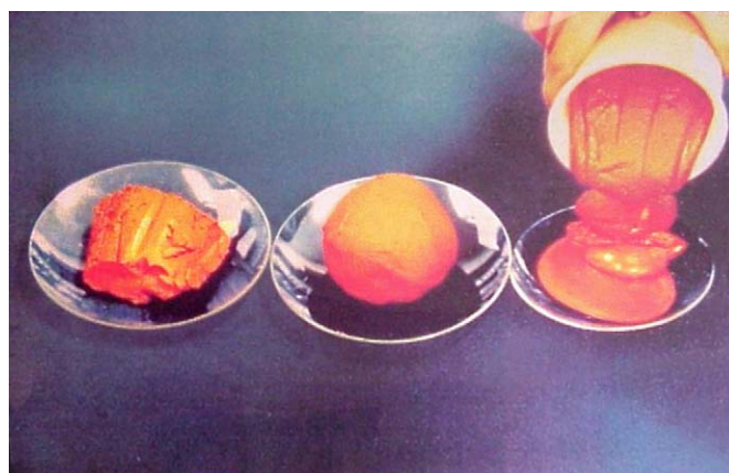
Fig. 2. Illustration of the effect of shear on a red mud filter cake.
